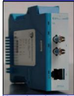
The 2E51 Media Converter Module provides fiber optic conversion to and from 10 BASE-T Ethernet to multi-mode optical power, conforming to the specifications of standards IEEE 802.3 and ISO/IEC 68802.3. The 2E51 does not require an EOTec 2000 power supply module for operation. Power connections located on screw terminals at the top of the module accept a nominal 24Vdc.
